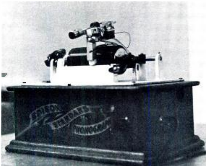
Edison phonograph for wax cylinder with a modified tone arm and Shure magnetic cartridge.
