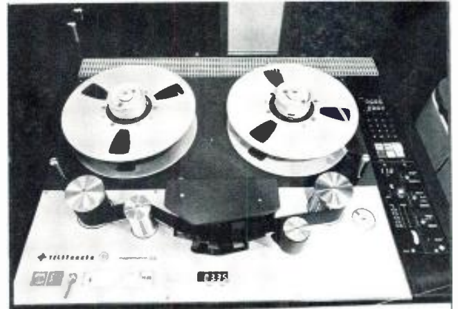
Telefunken's Magnetophon 15A transport. Note the vari-speed and auto locator modules on the right.
