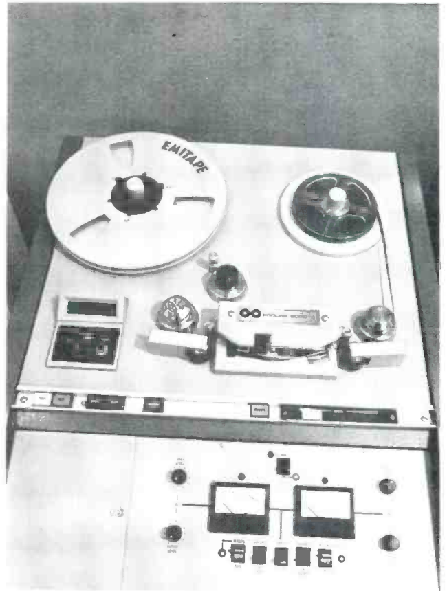
The Proline 2000TC, from Leavers-Rich. Note the dual capstan drive, and the tape position indicator to the left.
