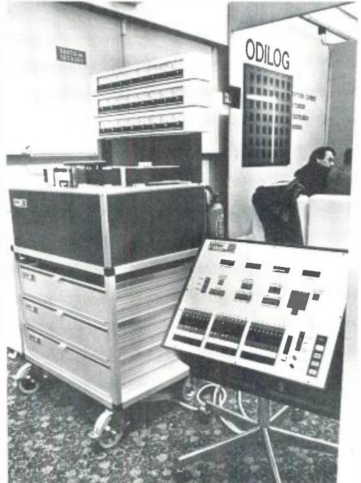
How's this for an auto locator? Lyrec's Tape Position Controller, with a 24 track machine in the background.
