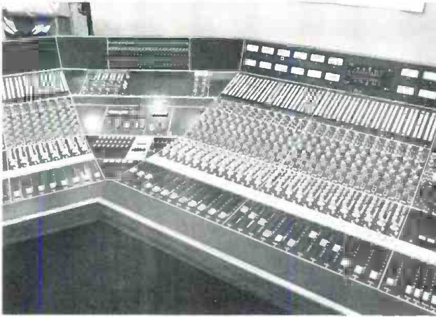
The Helios Electronic console for Maison Rouge Studio, London. The noise reduction panel is to the left of the meters.
