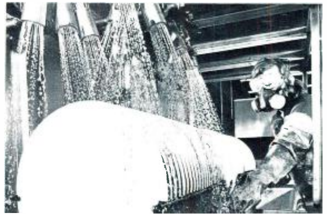
Figure 2. After being lapped perfectly smooth, the aluminum blank is etched and cleaned to provide a hospitable surface for lacquer coating. This is the final cleaning process.
