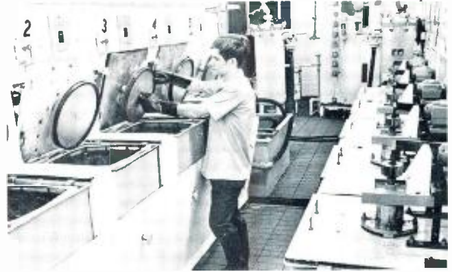
Figure 10. Mothers are made in these electroplating tanks. Plating is accomplished by the deposit of nickel on the surface of the master. This nickel mother is a positive of the original lacquer. It will be used to make the final mold, called a stamper, the reverse-image mold that actually is used to press discs. Many stampers can be made from a single mother.
