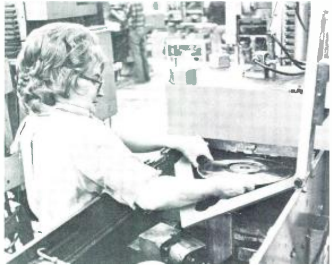
Figure 13. One of Capitol's many molding machines. A stamper is being inserted. During operation of the press, a biscuit of vinyl is extruded, labels are applied, and then the biscuit is pressed between two stampers, one for each side of the record, forming the final disc that will be trimmed, packaged, and sold at retail.
