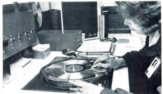
Figure 11. The nickel mother is played on special equipment. Minor groove problems can be corrected by manipulation of the groove wall with a pointed tool.
