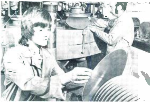
Figure 1. The new aluminum blanks are lapped on Capitol's specially designed machine seen in background.
