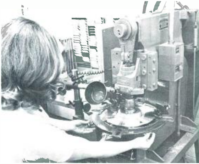
Figure 12. Once the stamper has been made, it is cleaned and trimmed and taken to the centering machine with which this worker will punch a center hole. To assure precision in the placing of that hole, she has a microscope equipped with a lined graticule. Following this operation, the stamper is back-sanded, die-punched, and formed to fit mold configuration requirements.
