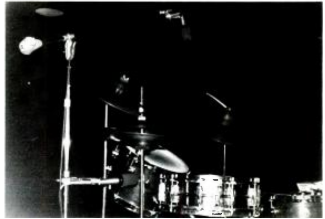
Figure 5. Two mics on drums—both sharing the same stand.
