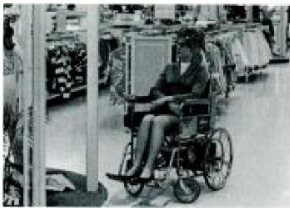
Figure 1. This motorized wheel chair is controlled solely by movement of the occupant's eyes. It is based on technology developed by space flight. Photo is courtesy of NASA.
