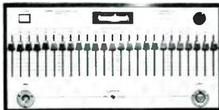
New B&K Model 124 Spectrum Shaper has 25 overlapping 1/3-octave bands with individual 40 dB attenuators to equalize audio system response curves from 56 to 17,500 Hz.
