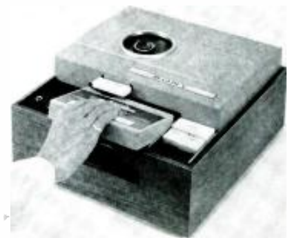
Figure 1. The Sony Videoplayer. The tape cassette will hold up to 90 minutes of videotape.
