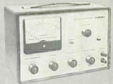
EICO 378 Audio Generator Switch selectable frequency output of 1 Hz to 110 kHz. Attenuated output in eight steps. Metered output voltage. Excellent frequency resettability. 0.1% distortion 20-20,000 Hz. $79.95
