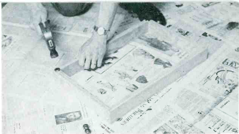
Furniture glides (which are not supplied with the kit) are most conveniently attached to base before it is screwed to enclosure.
