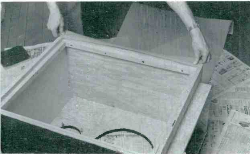
Grille cloth is measured to fit, and excess trimmed from edges.
