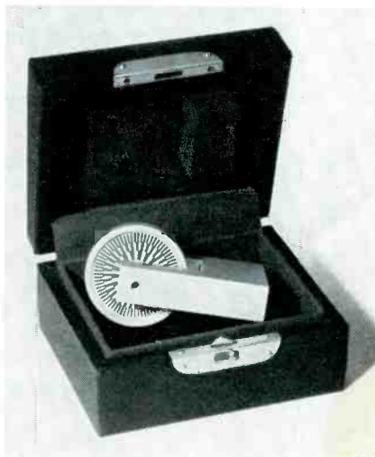
Strobe indicates proper recorder speed.
