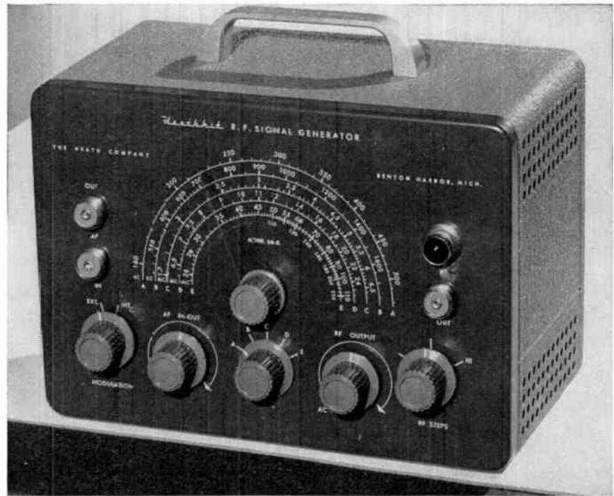
Fig. 2. Heathkit RF Signal Generator combines versatility with moderate cost.
