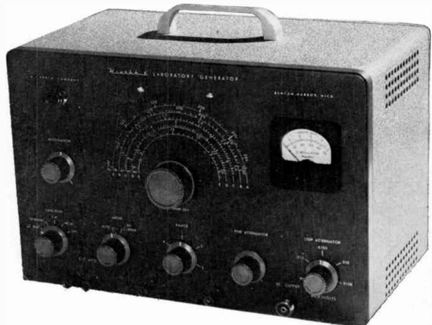
Fig. 3. Laboratory generator has refinements which adapt it to precision use.
