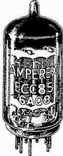
RF amplifier tube has internal shield.
