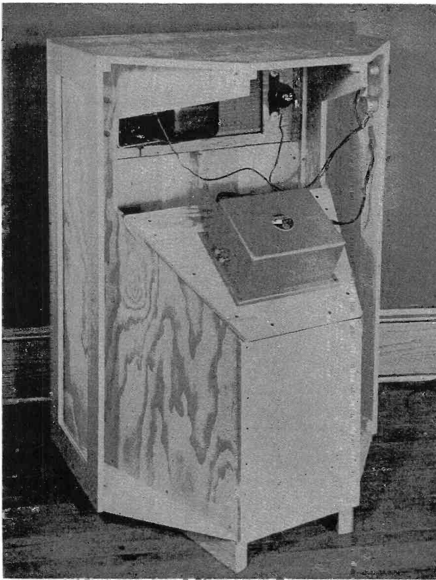
Kit completed except for grille cloth on wings. Note tweeter on front grille panel.
