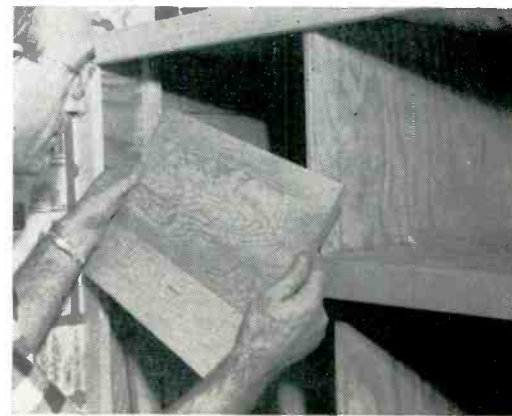
Fitting the amplifier control front panel.
