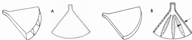
Fig. 12—A, sectoral horn; B, diffraction horn.
