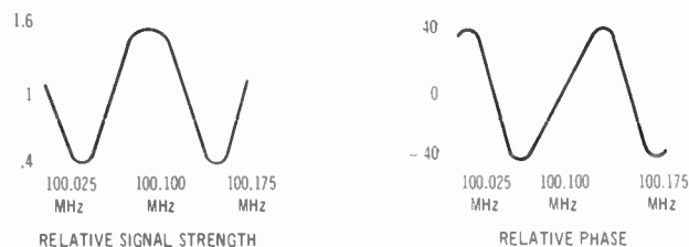
Fig. 3c—Amplitude and phase response of total transmission path containing one reflection.
