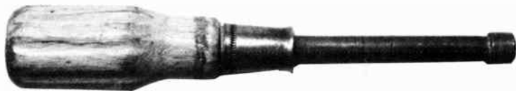
Fig. 4—A nutdriver used with a screwdriver helps assembly of hard-to-get-at screws and nuts.
