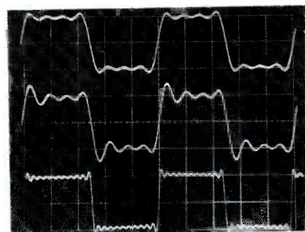
Fig. 3—Square-wave response for 3 kHz into 8-ohm load (top), 3 kHz into 8 ohms paralleled by 2 μF (middle), and 22 Hz into 8 ohms (bottom).
