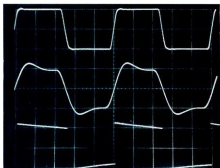
Fig. 2—Square-wave response for 10 kHz into 8-ohm load (top), 10 kHz into 8 ohms paralleled by 2 \mu F (middle), and 40 Hz into 8 ohms (bottom).
