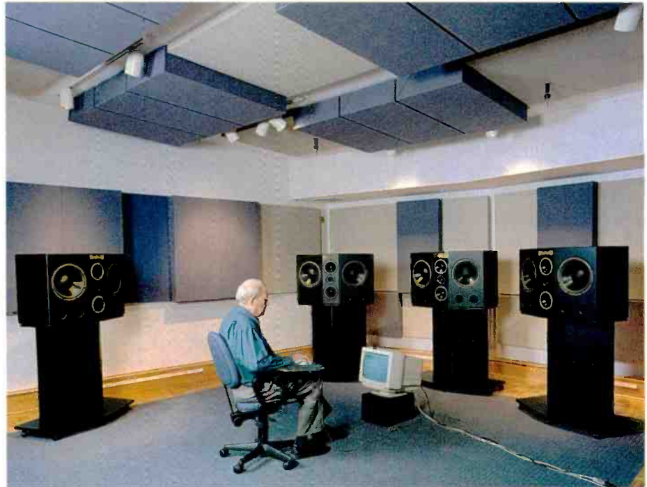
FIG. 2— Evaluation laboratory at CRC, where behavioral scientist Ted Grusec (seated) conducts scientifically controlled listening tests. The speakers are professional monitors made by State of the Art Electronik, in Ottawa.
