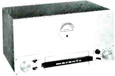
Classic '50s high end: The Marantz Model 9 tube power amplifier had adjustable bias, DC balance, and AC balance.
