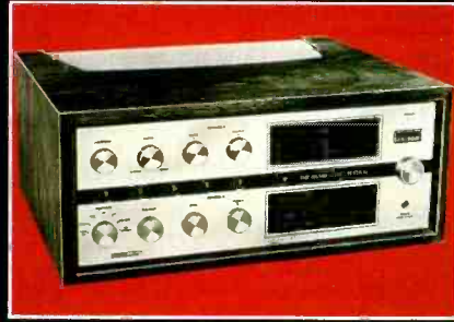
Among the earliest stereo receivers, this Harman Kardon Festival model had duplicate controls for each channel and separate dials for FM and AM tuning.
