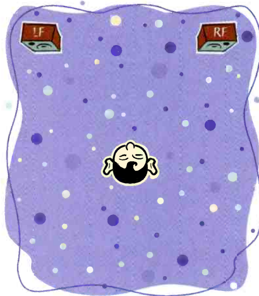
Fig. 1—Because of the stereo-seat restriction, two-channel stereo is an antisocial system; only one listener at a time can hear it properly.
