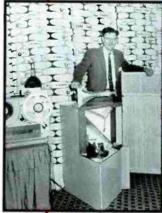
Paul Klipsch's folded-horn speaker, the Klipschorn, could produce deafening sound levels from low-powered '50s amplifiers.
