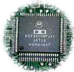
B&K's new surround sound components are powered by the 24-bit Motorola 56000 DSP.
