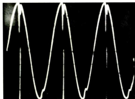
FIG. 2 —PROTECTION-CIRCUIT SPIKES IN TWO OTHER POWER AMPLIFIERS.
