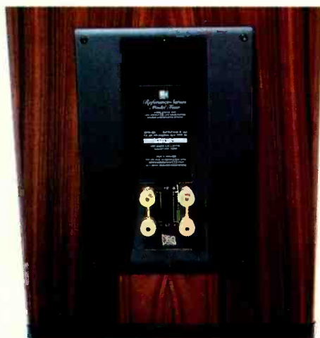
The terminals allow bi-wiring and are easy to reach and grip, but they won't accept double-banana plugs.
