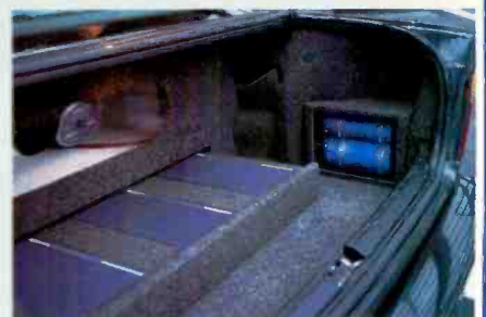
Amplifiers and subwoofer compartment, with capacitors in background.
