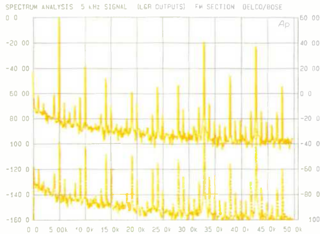
Fig. 6—Spectrum analysis of crosstalk and subcarrier products for FM stereo signal with one channel modulated by 5 kHz (solid curve) and other channel unmodulated (dashed curve). Scale at right is for bottom curve.
