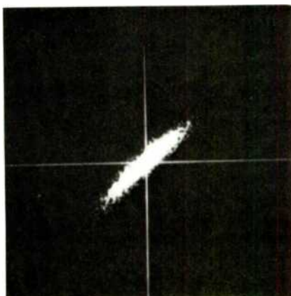
Fig. 6— Interchannel phase difference of arm/cartridge using pink noise from B & K 2011, band 7.
