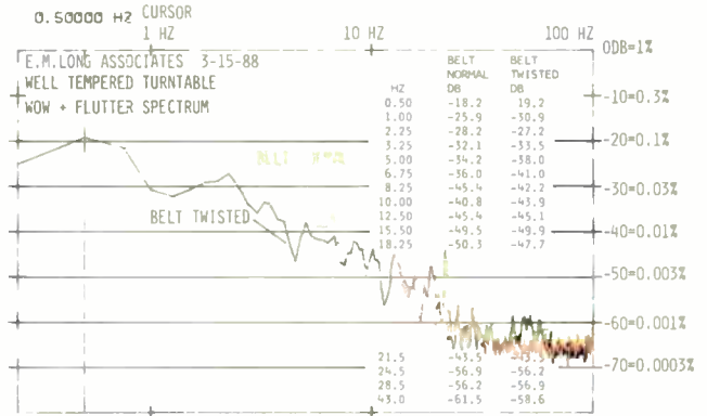
Fig. 2—Wow and flutter spectrum, from 0 to 100 Hz. Note the improvement in performance with the belt twisted (see text). The arm cartridge resonance with the van den Hul
