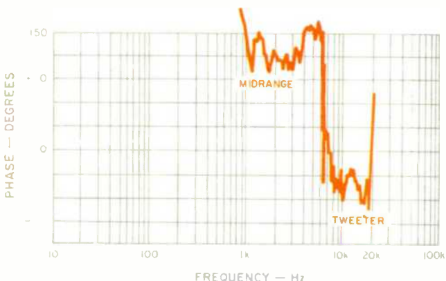
Fig. 5—Free-field phase response at 3½ meters. The midrange response is corrected for 11,980- \mu S time delay, while the tweeter response is corrected for 10,308- \mu S time delay.
