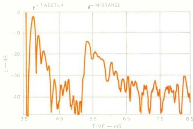
Fig. 8—ETC of Fig. 7 with an expanded time scale and corrected for a 1-meter measurement position.
