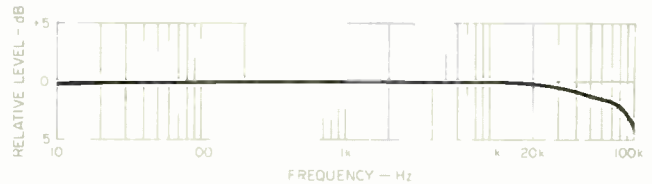
Fig. 6—Frequency response at 1 watt output into 8-ohm load.
