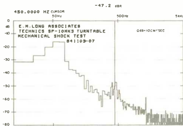
Fig. 7— Spectrum to 5 kHz due to mechanical shock applied to the massive platform upon which the turntable and base rested during tests. Resistance to such shock was very good.
