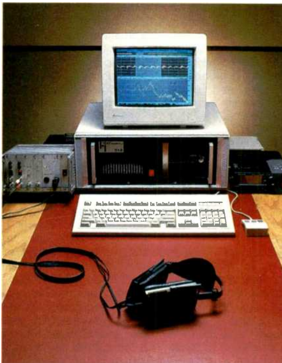
Head Acoustics binaural analysis system with keyboard and mouse (center), flanked by Reproduce Unit for electrostatic headphones (left) and specially modified DAT recorder (right).
