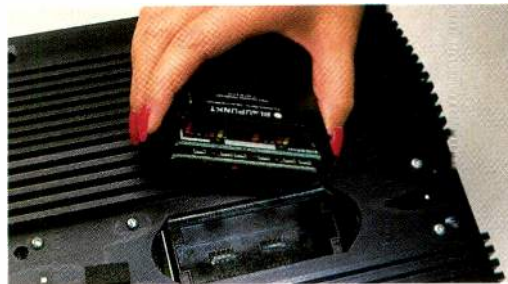
Lifting the Blaupunkt's top trim plate reveals the socket for its custom equalization module.
