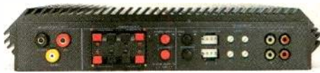
Terminal side of the Altec Lansing ALA-435, showing (left to right) power and control terminals, home-type speaker terminals, bridging switches, high/low input-select buttons, high-level input terminals, individual-channel level controls, and RCA-type audio inputs.
