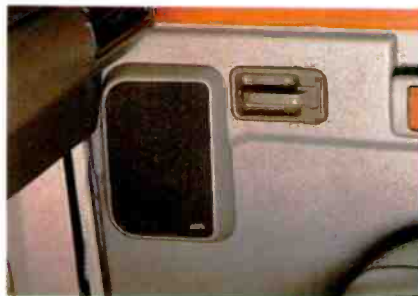
This wedge-shaped Z-Box enclosure looks like factory stock but positions the new speaker for clearer response and better imaging.
