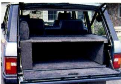
The sound system cabinet (at right of trunk) infringes on trunk space less than the factory-supplied panel that covers the spare tire (left).
