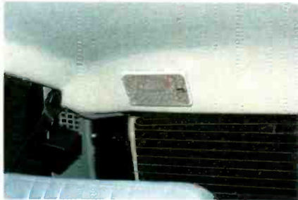
The new rear speakers were mounted in the car's original enclosure.
