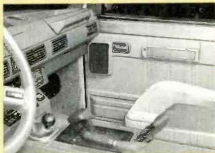
Front speakers, including a/d/s/ S7 woofer in kick panel below dash and 200i system in Z-Box enclosure on door.
