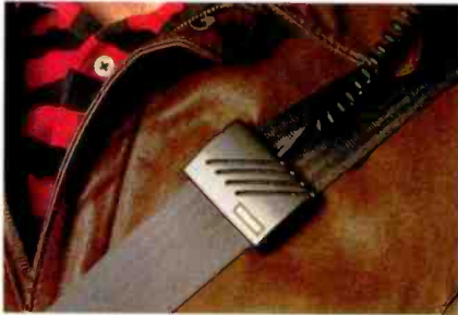
Shure microphone, clipped to shoulder belt, was used for hands-free telephone calls.
