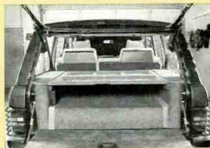
With the parcel shelf in place, the system enclosure cramps the trunk space.
