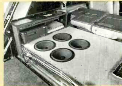
Subwoofer enclosure and left side cabinet. Note crossovers, fan, and S7 woofer set into cabinet top, and Alpine 5950 changer and a/d/s/ PQ20 amp on shelf.
