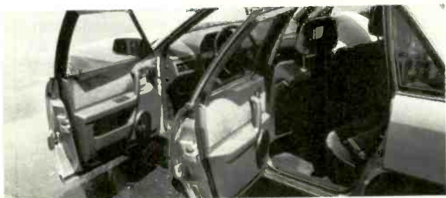
This unusual installation features three-way 763 component systems in front, with 6 1/2" subwoofers installed in doors, Varimount® tweeters surface-mounted on doors, and 4" midranges in dash. 767 6 1/2" two-way uniaxial systems in rear doors.
