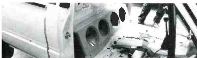
(Left) 741 system in rear of cab. Includes 1" Varimount tweeter (above) and 4" woofer (below). (Right) Varimount tweeter under headliner.
