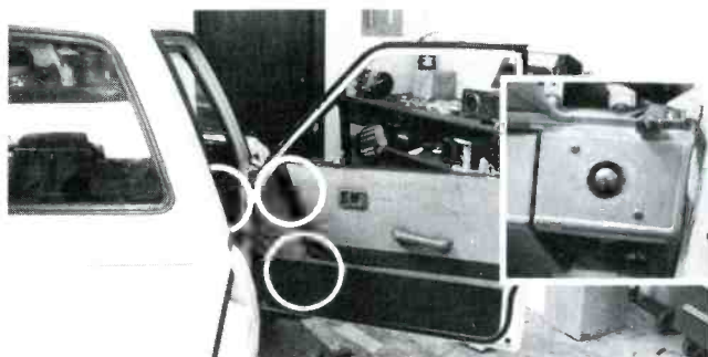
View from rear of truck. The two circles on the door show location of 761 system (1" Varimount tweeter, above, and 6 1/2" woofer below). The half circle at left shows dashboard location of 701 tweeter. (See insert photo.)
