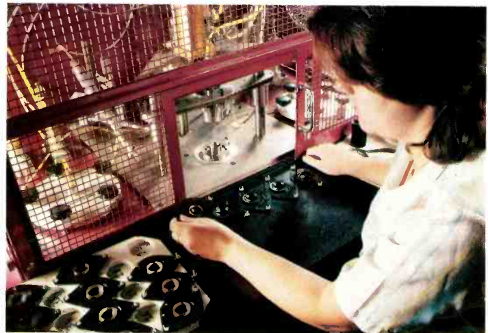
B&W's automated tweeter assembly. Technology in the service of music.
