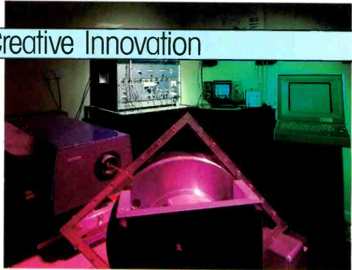
Dr. Glyn Adams, head of B&W's research department, pioneered a technique for monitoring the vibrational behaviour of loudspeakers using lasers.
