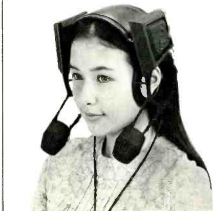
These prototype JVC headphones included a second pair of drivers in front of the listener's ears to enhance frontal localization.
