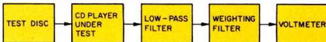
Fig. 1—Test setup for measuring S/N ratio, as recommended by the EIAJ. Using a "low-pass" filter (see text) eliminates all out-of-band noise from the measured results.
