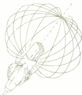
Fig. 23—Three-dimensional representation of supercardioid polar pattern.
