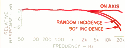
Fig. 13—High-frequency roll-off due to case diffraction, omnidirectional microphone.
