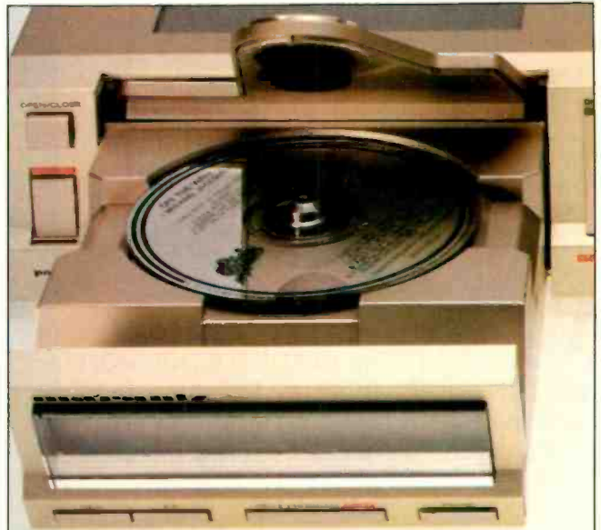
When the "Open/Close" button is touched, the disc drawer slides out and the door's front face swings down by 45°.
