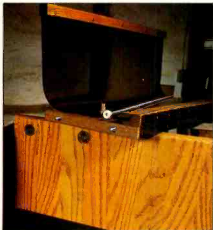
Pins on Barzilay lid engage holes in cabinet sides. Threaded rod is Naiad's compression fitting.
