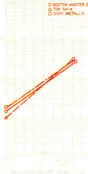
Fig. 4— Third-harmonic distortion vs. level at 1 kHz with Dolby C NR.
