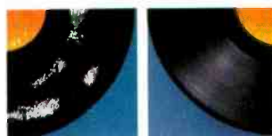
(Left) Foam beads are attracted to static charge left on record after cleaning with a leading record cleaner. Same record (right) after one treatment with Sound Life fluid with anti-static action.
