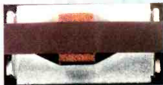
TDK dual spring pressure pad and tape in cassette.
