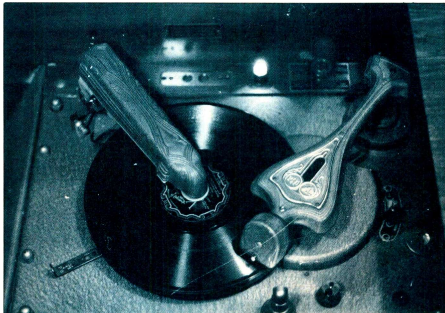
RCA Victor's Duo was made from 1931 to 1937. Note huge pickup head.
