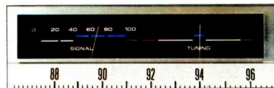
SIGNAL STRENGTH AND CENTER TUNING METERS FOR A DRIFT-FREE PERFORMANCE.
