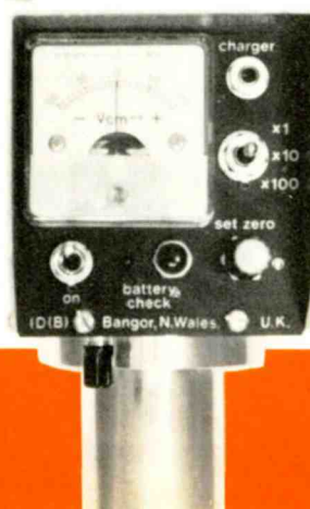
Fig. 2 — Meter on rear of field mill test instrument reads directly in volts/cm and also indicates polarity of the static charge.
