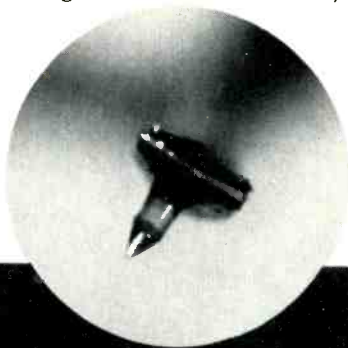
Fig. 11a—No lint on the stylus tip.
