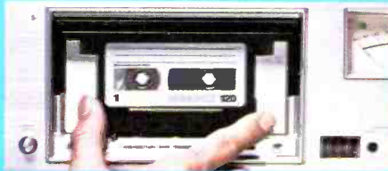
Simple vertical cassette insertion visible at all times.
