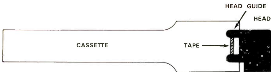
Fig. 2—An accurately aligned head guide will position the tape exactly in the center of the cassette, as shown here.
