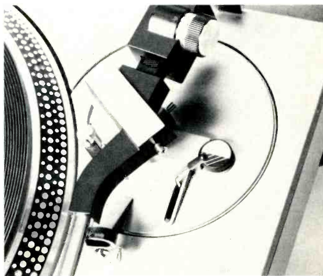
Fig. 2—Close-up of arm mounting showing balance and stylus-force adjusting knob, cue control, anti-skating control, and arm lock.
