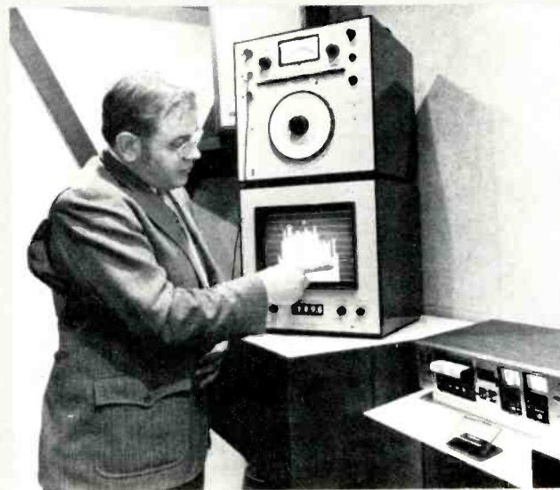
The B&K 1/3-Octave Analyzer display indicates the peak music at each 1/3 octave. Top photo shows display with Scotch brand High Output Low Noise tape. Bottom photo shows display with new Scotch brand Special High Performance tape, which was found to be better than 10 dB over regular tape at 16 kHz.
