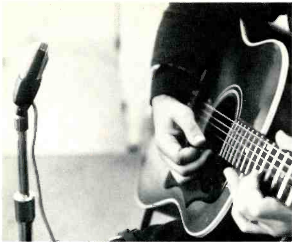
Fig. 3 —Acoustic guitar pickup using a bidirectional velocity mic, in this case the RCA SK-66. Most velocity mics have a bass rolloff of some sort, either fixed or variable, that can be used to counteract the proximity effect to be expected when the mic is used this close.
