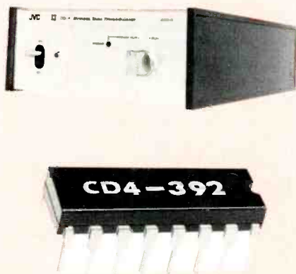
Fig. 3—Two of these ICs, plus a few small components, can replace JVC's 4DD-5 unit above.
