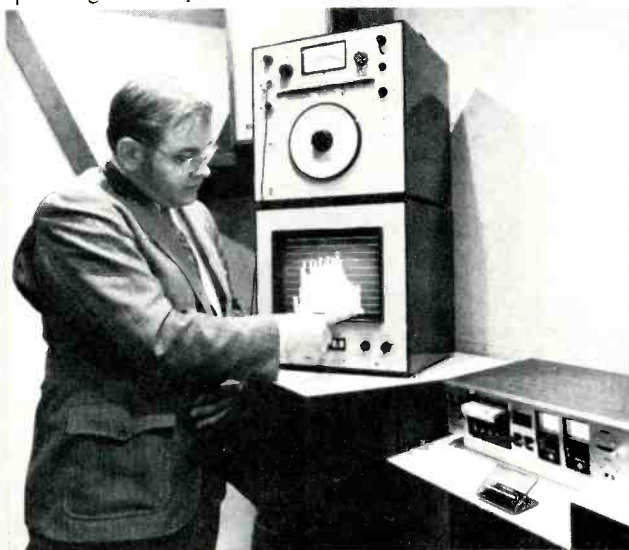
The B&K 1/3-Octave Analyzer display indicates the peak music at each 1/3 octave. Top photo shows display with Scotch brand High Output Low Noise tape. Bottom photo shows display with new Scotch brand Special High Performance tape, which was found to be better than 10 dB over regular tape at 16 kHz.
