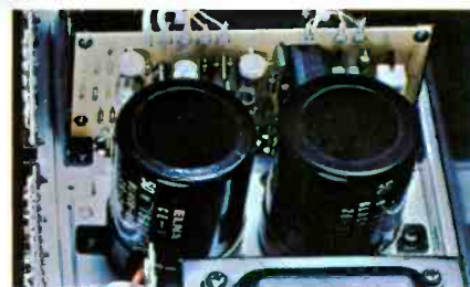
Two 15,000uF power supplies eclipse anything now available in integrated amplifiers.
