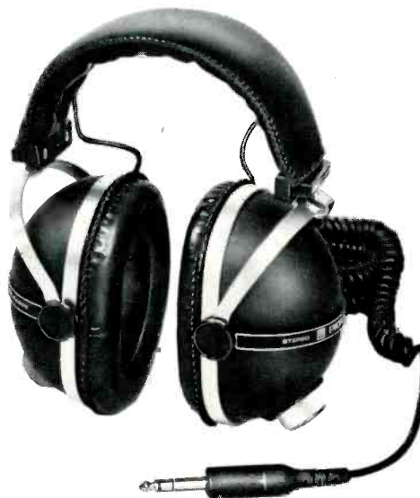
Fig. 3—These 8-ohm phones, Pioneer SE-405s, can handle 500 mW; require only 11.25 mW to produce 113
