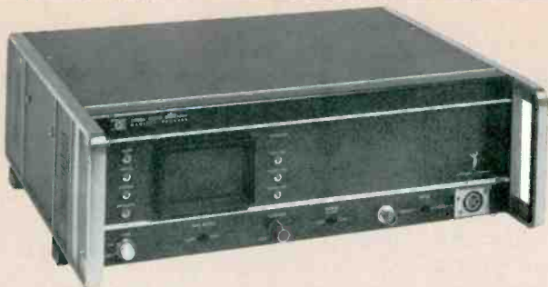
Fig. 3—The 8050A Real Time Analyzer, a device which provides continuous monitoring of sound energy levels in one-third octave bands. The response, which is updated each 30 milliseconds, can be viewed in either fast or slow modes.
