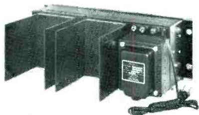
Advanced design heat sink provides protective cooling.
