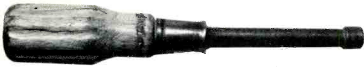
Fig. 4—A nutdriver used with a screwdriver helps assembly of hard-to-get-at screws and nuts.
