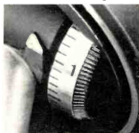
Stylus pressure dial calibrated in tenths of a gram from 0 to 1.5 grams; in quarters of a gram from 1.5 to 3.0 grams.
