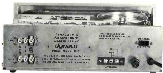
Fig. 1—Rear panel layout of the Dynaco FM-5
