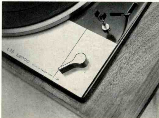
Fig. 2— ON/OFF switch at the right-front corner of chassis, with the arm rest just back of it, followed by the cueing lever.
