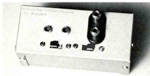
Fig. 1 —Exterior view of battery-operated preamp used to provide sufficient gain for use in turntable measurements. Since this photo was taken, another switch has been added to place a 10- \mu F capacitor in the feedback circuit to give flat response.
