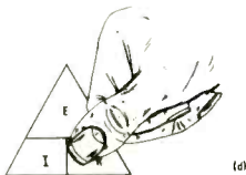
Fig. 9—Ohm's law. The triangles are a memory aid for remembering the various forms of the law. Ohm's law triangle (a). Drawing (b) shows how to determine voltage. Cover E with a finger and the answer is I \times R . In (c) I = E/R and in (d) R = E/I .
