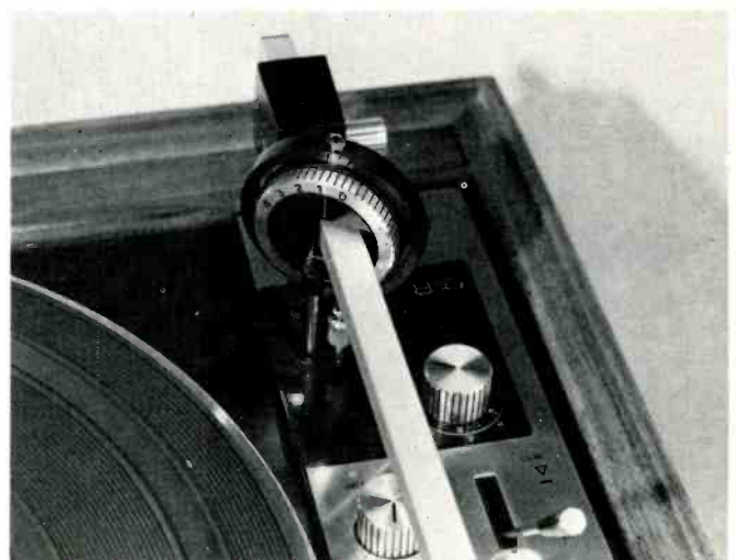
Fig. 2—The arm-mounting gimbal has the anti-skating control at its right and the set-down control directly in front. Stylus force is set by the large ring on the gimbal. The cue lever is shown at the right front.
