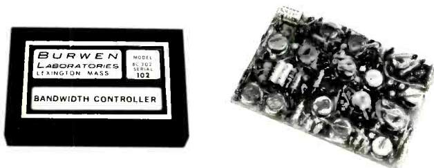
Fig. 5—A high performance module incorporating 15 operational amplifiers.
